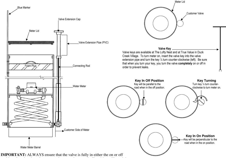
**IMPORTANT:** ALWAYS ensure that the valve is fully in either the on or off position. Leaving the valve partway between the on and off position will result in water running through the stop and waste valve, which registers as usage on your meter. This will result in high water charges on your bill.
